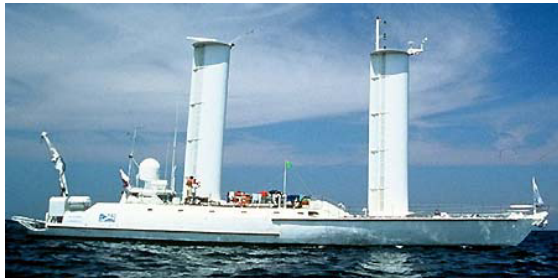
Figure 4: Commandant Cousteau's Alcyone fitted with its suction airfoil of type Turbosail
