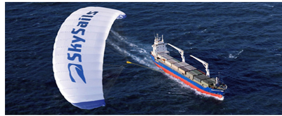
Figure 10 : Cargo ship propelled by a dynamic kite (image SkySails)
