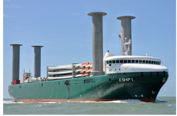
Figure 8: E-SHIP 1, fitted with four Flettner rotors
